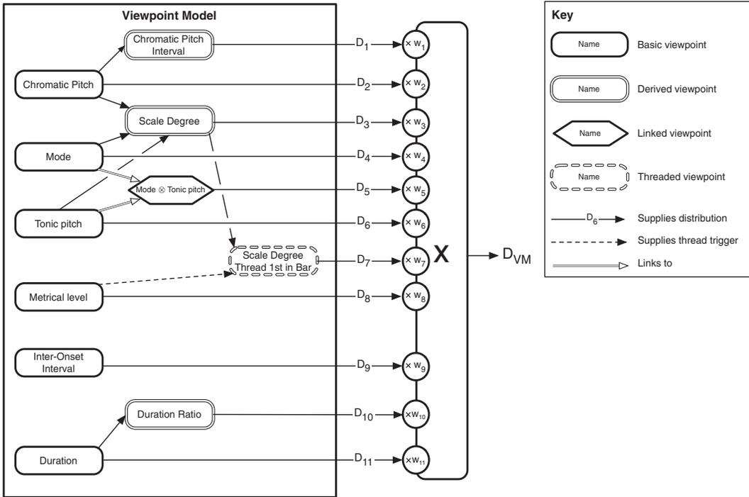
Fig. 2. Schematic diagram of the viewpoint models, showing a subset of available viewpoints.  $D_i$  are distributions across the alphabets of viewpoints,  $w_i$  are the entropic weights introduced in Section 3.3, and  $D_{VM}$  is the overall distribution derived from the combined viewpoints.
