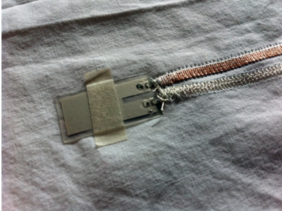
Fig.15: Wiring with copper tape.
