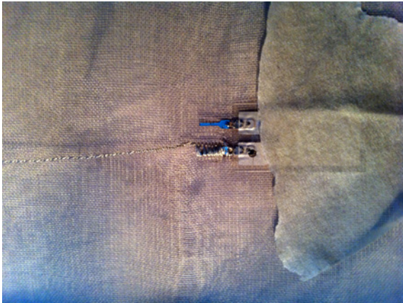
Fig.13: Sewing the piezo film with silver thread.
